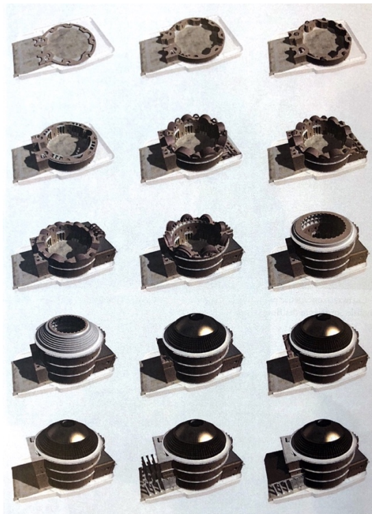
“Visualization of the sequence of operations in building the Pantheon.” (Marder & Jones, 2015, ‘Plates Section’ 204)
