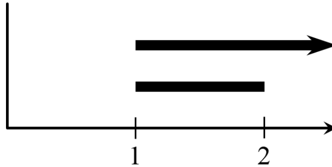
Figure 5.6: The barcode in dimension 1 of the filtration presented in Example 5.1. Each bar in the barcode represents the birth and death of a homology class in the filtration. Note that the complex contains a 1-cycle which is born and dies at 2, so it does not appear in the barcode.
