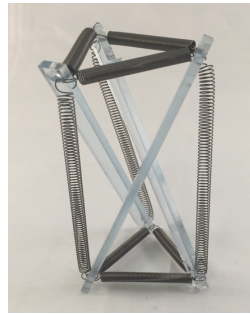
(c) The final form of the constructed tensegrity.
