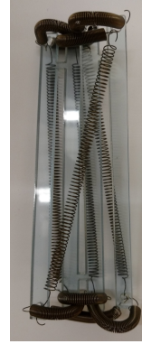
(b) The constructed tensegrity before the struts are separated.
