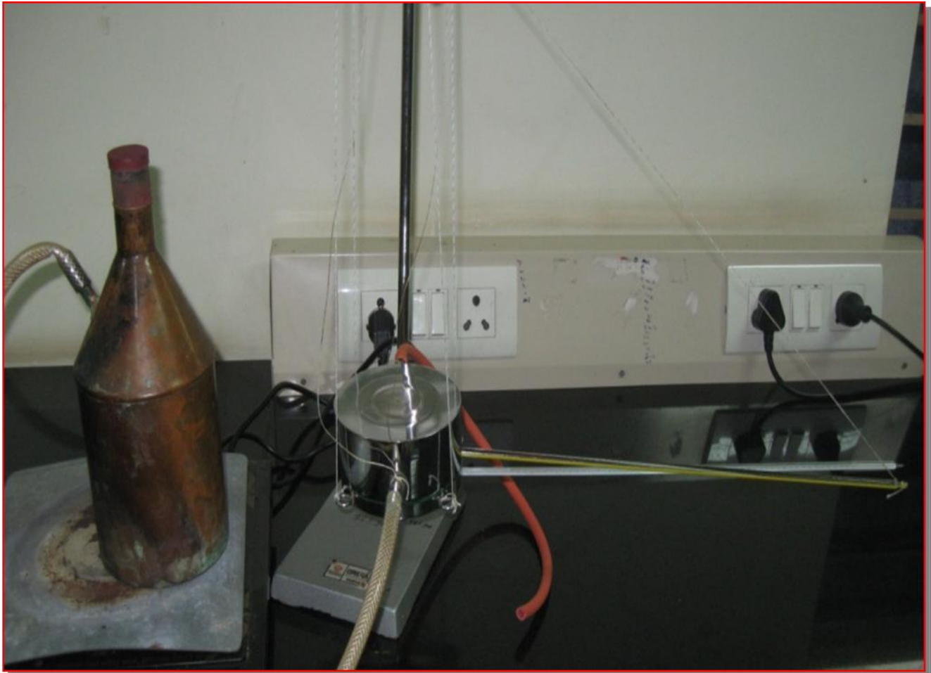
Plate 4: Photograph of thermal and electrical conductivity measurement setup
