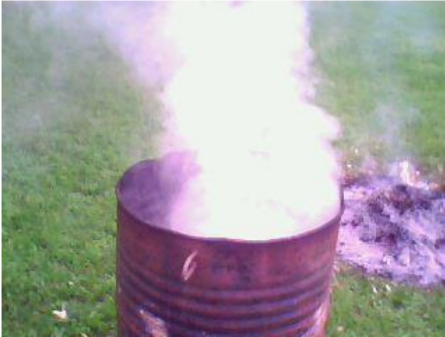
Plate 1: Bamboo Leaf Ash Burnt in an open Atmosphere
