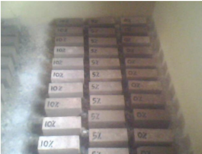
Plate 4: Picture of block samples produced with the BLA blended cement arranged on the floor of the laboratory undergoing curing.
