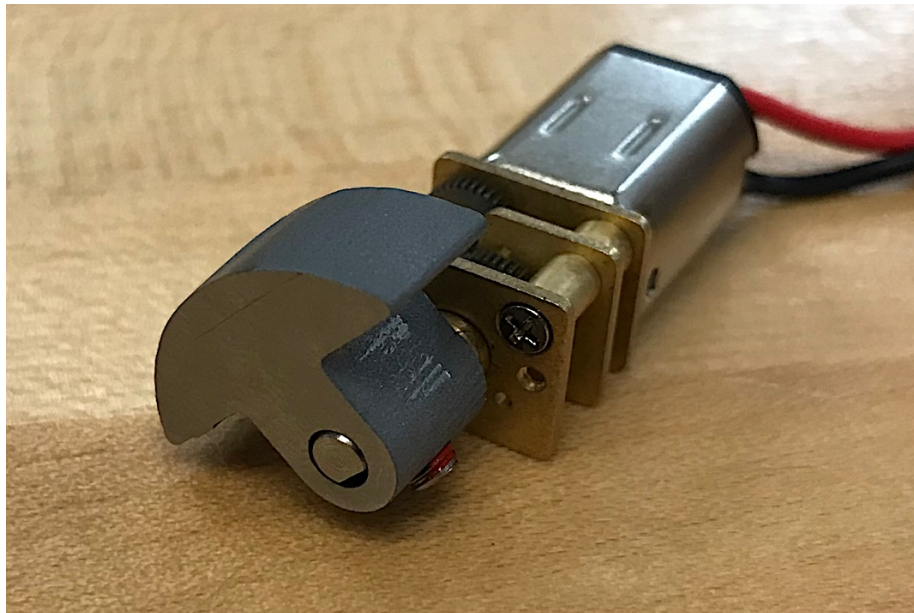
Fig.13 – Pololu 10:1 Micro Metal Gearmotor LP 6V equipped with custom eccentric weight
