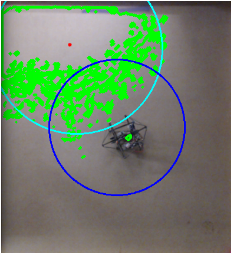
Figure 7: An example of how a change in lighting can mess up the tracking software. In this picture, the hallway light had previously been off but turned on when someone was walking down the hall, causing a bright patch which threw off the tracking code.
