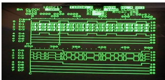
Gambar 5. Hasil Pengujian proses Spreading-Despreading PN-Code Gold [5,3]-[5,4,3,2].
