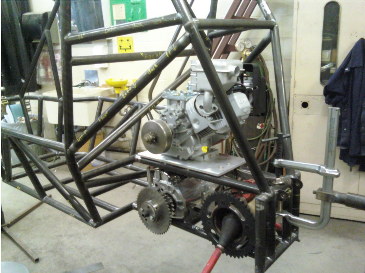
Figure 24: Fabricated Drivetrain and Framing
