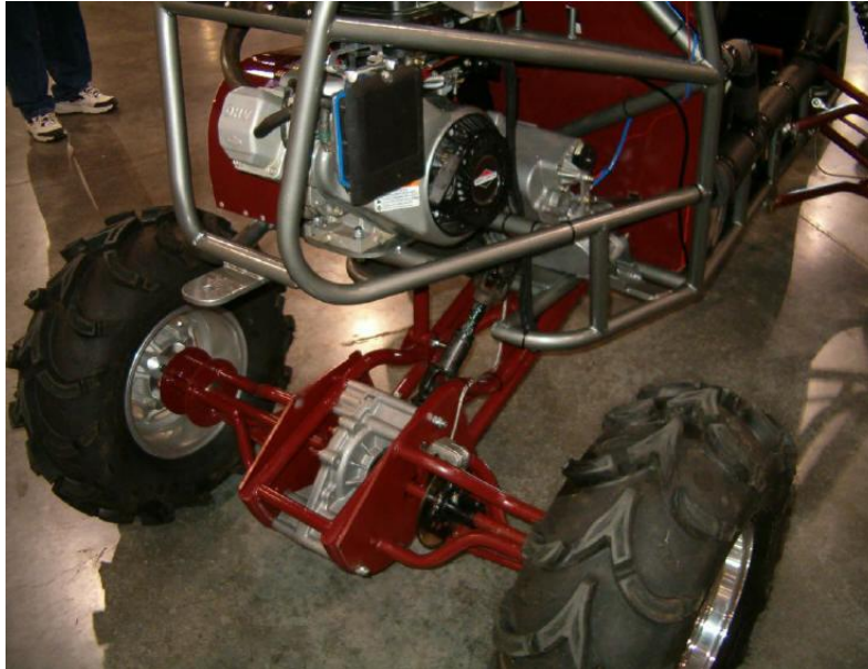
Figure 6: Swing Arm Style Suspension
