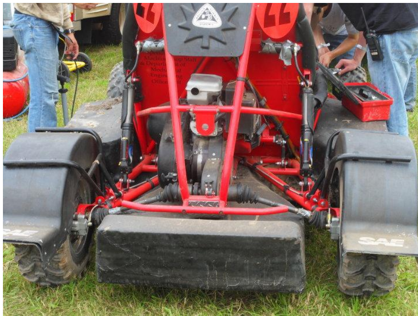
Figure 2: Picture of drivetrain, rear suspension, and rear framing
