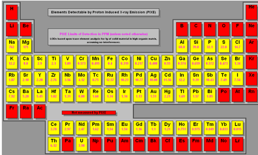
Figure 1: The elements detectable and the minimum detectable limits for PIXE in ppm [2].
