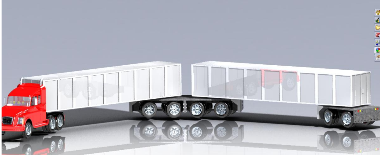
Figure 2.2: A view of a single bogie. The bogie is attached to the trailer with the same 5 th wheel coupling found on the tractor. This allows the bogie to pivot. To attach this, the trailer owner can simply cut off the existing bogie wheels and weld on the new coupling.
