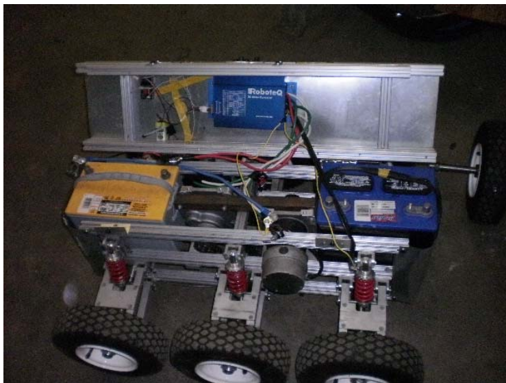
Figure 3.10: The drive system installed.
