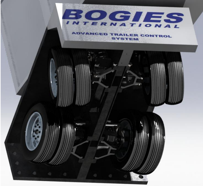
Figure 2.2: A view of a single bogie. The bogie is attached to the trailer with the same 5 th wheel coupling found on the tractor. This allows the bogie to pivot. To attach this, the trailer owner can simply cut off the existing bogie wheels and weld on the new coupling.
