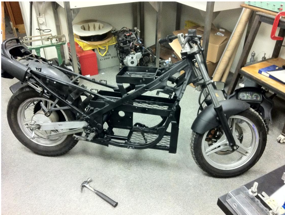
Figure 22: Final modified motorcycle chassis
