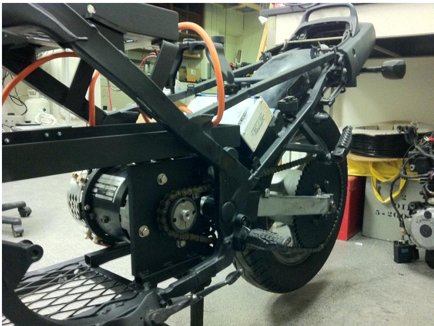
Figure 19: Chain and sprocket drive train final configuration
