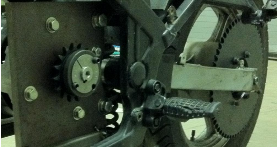
Figure 18: Direct drive sprockets
