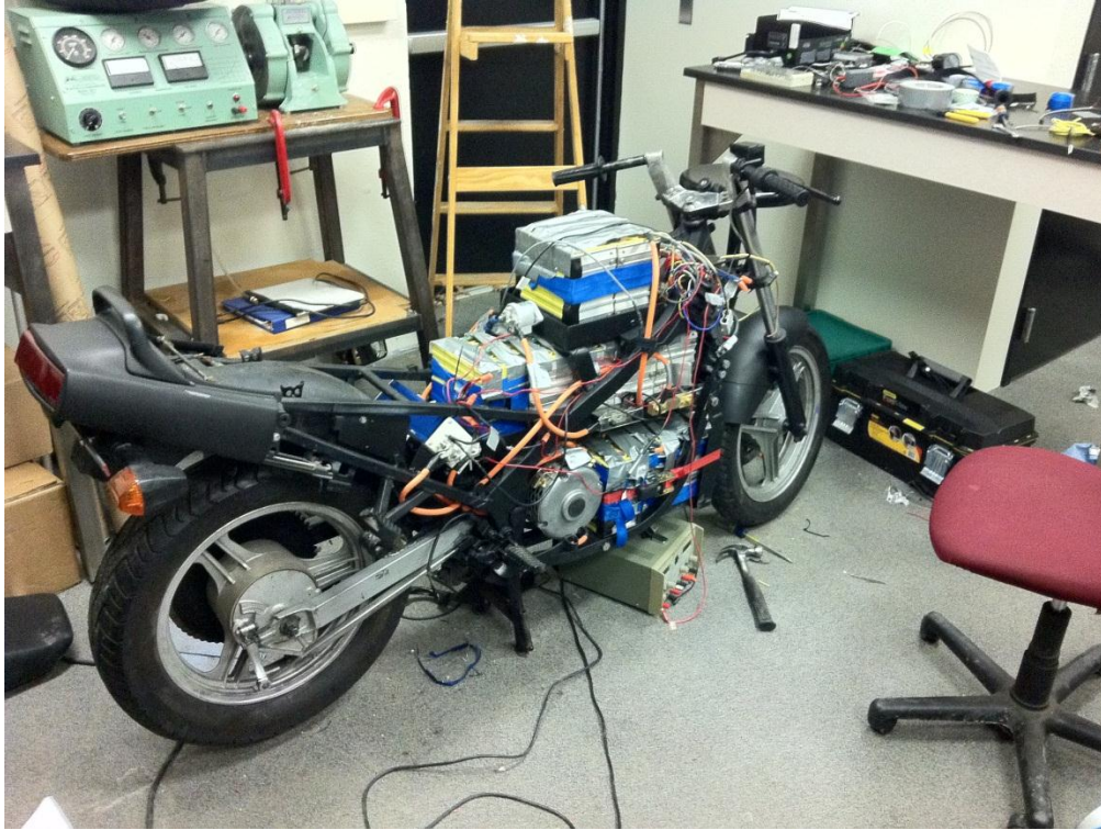
Figure 23: Completed drive system mounted to project bike
