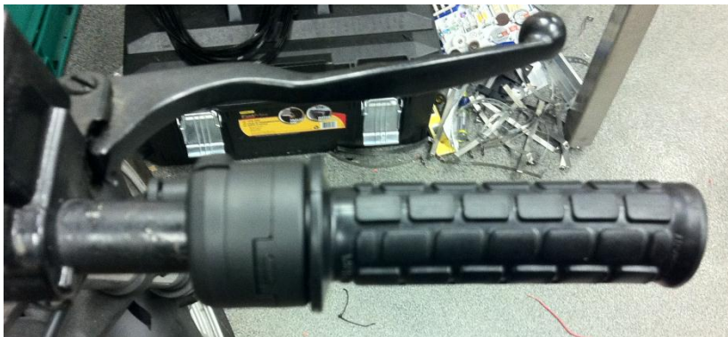
Figure 15: Twist grip style potentiometer
