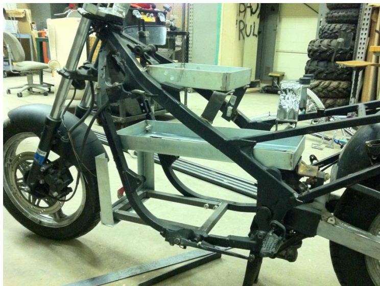
Figure 6: Battery Mounting Trays
