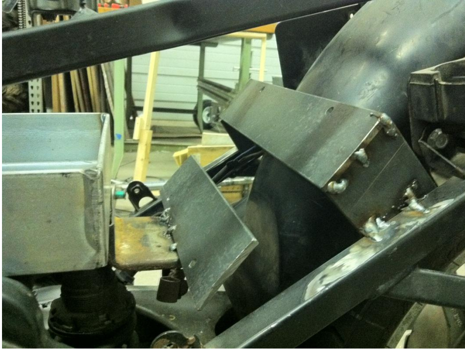
Figure 16: Motor controller mount in its location on the motorcycle chassis
