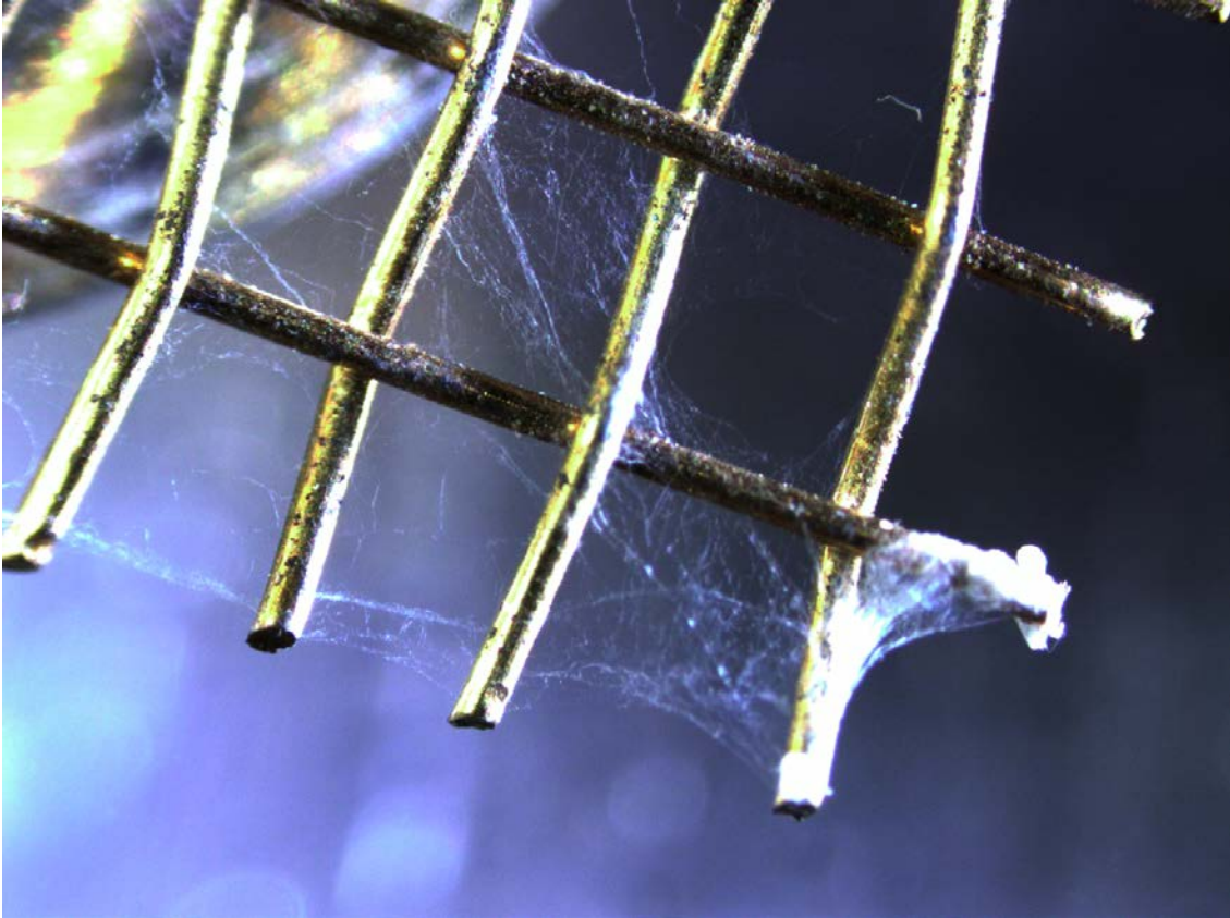
Figure 3: Electrospinning results achieved with a chloroform polymer solution. These fibers are on the micrometer scale.
