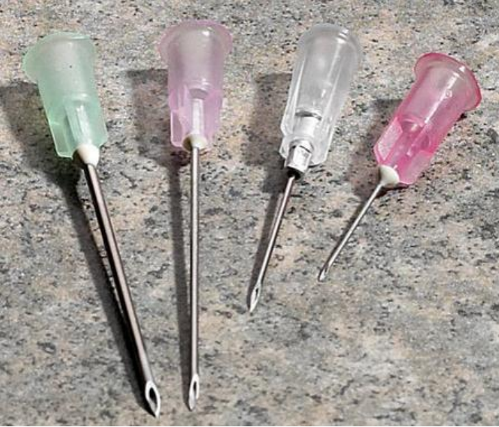
Figure 13: The needles used in the lab. On the left is a 19 Gauge needle and on the right is a 30 Gauge needle. (Courtesy of James Maher)
