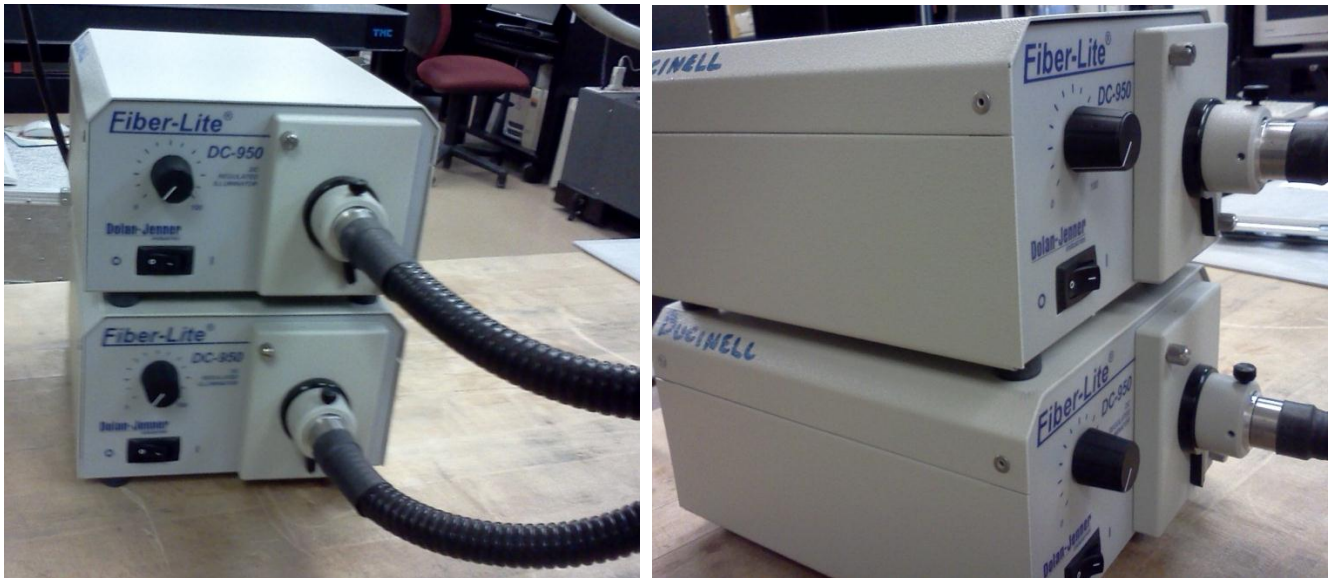
Figure 6: The fiber lights source providing cool lights used during an experiment.
