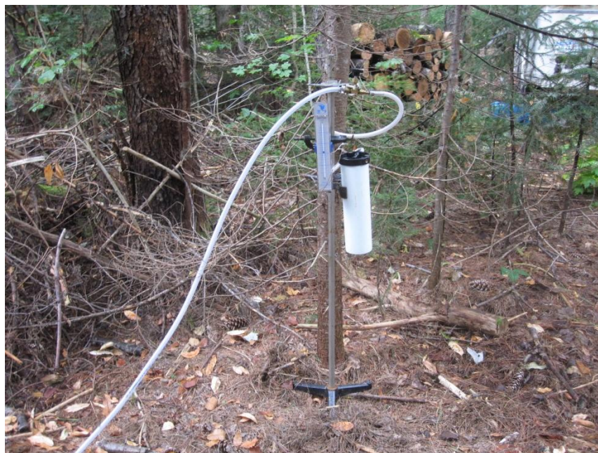
Figure 4. The impactor, encased in a white protective shell, is mounted in the woods at the Piseco Lake site.
