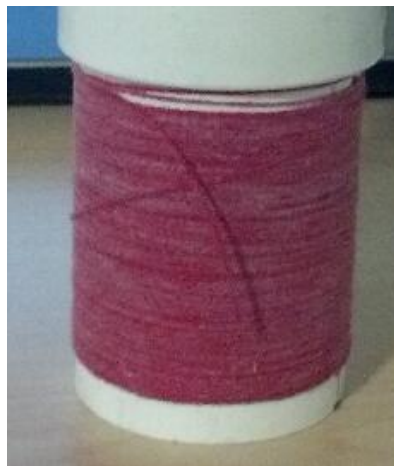
Figure 20. The spooled yarn that has been coated with aerogels. Note the slight discoloration (white tint) due to the aerogel material.
