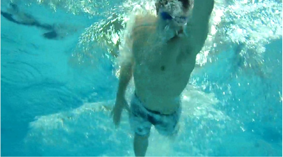
Photograph of the bottom view of the 50% MTMS Aerosuit in use. The air bubble surrounding the suit is very visible from this angle. Bubbles created by the swimmer have similar reflective properties as the bubble enveloping the suit.
