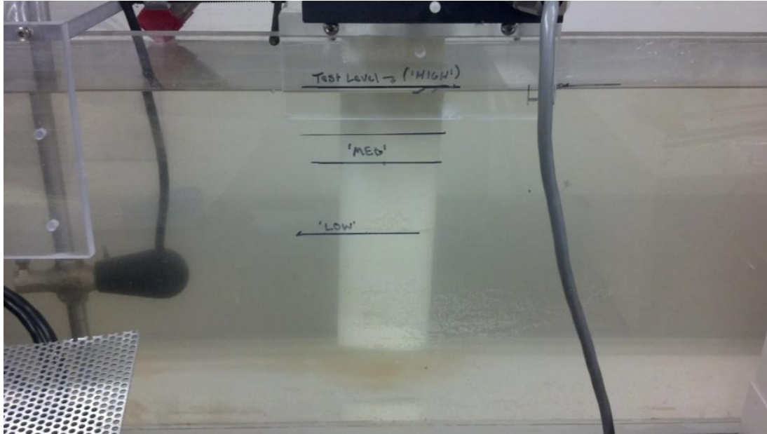
Figure 29. The filled test section of the water channel with the airfoil inside of it and connected to the dynamometer. This setup was used for drag testing. Water was held at this constant level.
