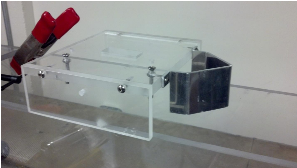
Figure 15. The dynamometer mount with the blocker added.
