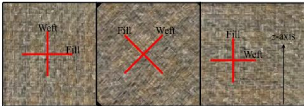
Figure 5. Left: BL fabric at 0^\circ (weft is parallel to the z -axis). Center: BL fabric at 45^\circ . Right: BL fabric at 90^\circ (weft is orthogonal to the z -axis).
