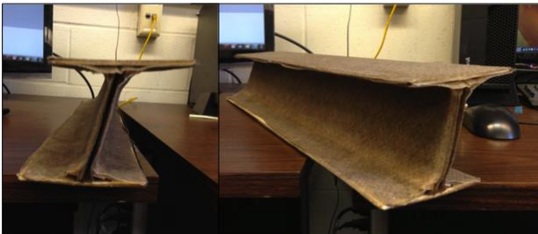
Figure 17. Two views of the first I-beam are shown. Note the non-vertical orientation of the web.
