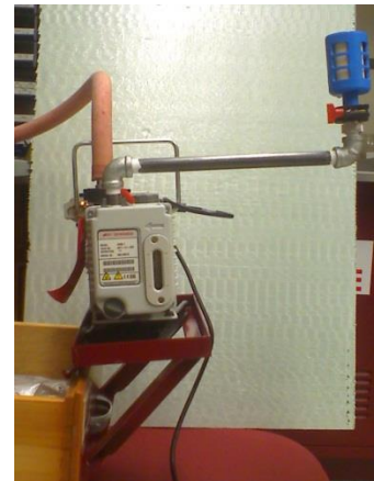
Figure 5.3 Mock-up of modified gas pump with stand
