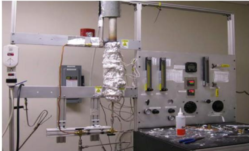
Figure 2.4 The current catalytic test bed. The probe for the 5 gas analyzer is hanging on the left side of the frame beneath the detector. The emissions blend tank is located to the right of the image.
