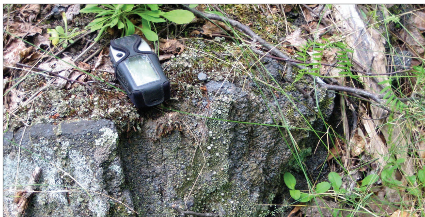
Figure 2: Outcrop of the magnetite-fluorapatite ore. The 4 inch GPS device is for scale.
