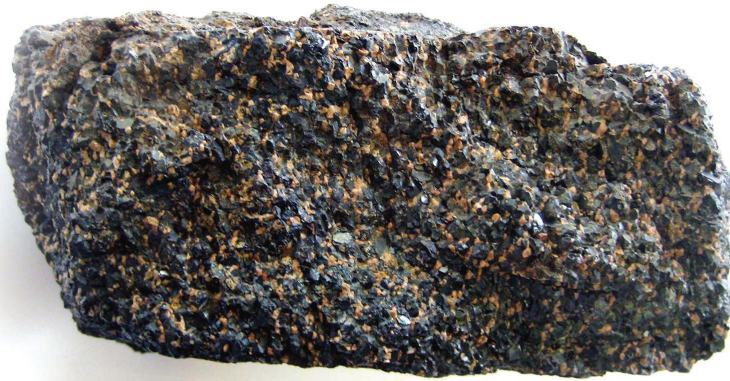
Figure 1: Hand specimen of magnetite (dark)-fluorapatite (light orange colored) ore from Mineville.
