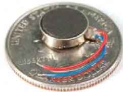
Figure 10: A vibration motor that could be attached to a real life soft robot to generate locomotion.
