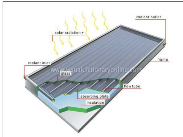
Figure 1: Flat plate solar collector. [6]
