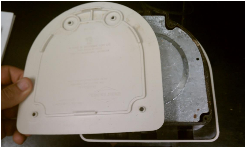
Figure 11: First Step of the Popper Disassembly
