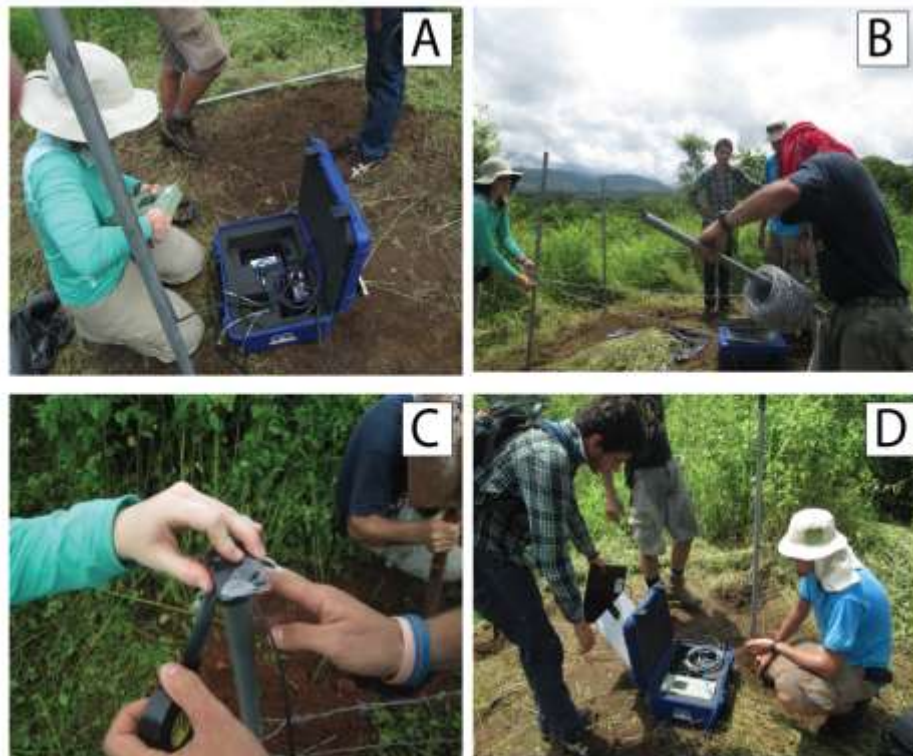
Figure 12. Additional seismic station setup. (a) Digitizer hook-up to seismograph and battery. (b) Fence built around station to protect against outside disturbances. (c) GPS taped to fence post to record accurate time. (d) Final setup in blue protective casing, with solar panel attached on top.
