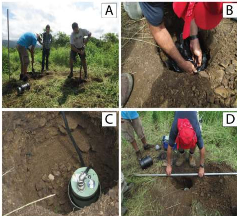
Figure 11. Initial steps involved in setting up the seismograph in the ground. (a) Digging a 0.5-1m hole to bury the seismograph. (b) Covering the seismograph with plastic to protect against water damage. (c) PVC casing placed around seismograph to secure it in place. (d) Aligning seismograph towards north.
