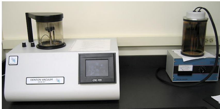
Figure 7. The Denton Vacuum deck IV standard Sputter Coater at Union college [7].
