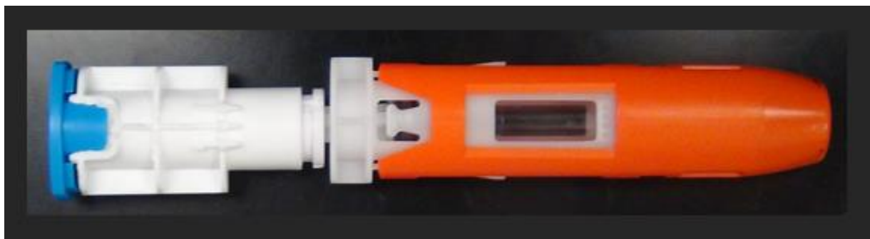
Figure 7: EpiPen® with outer casing removed and the blue safety still installed. The main compressive spring has been removed and not replaced in this image. The blue safety cap remains installed locking the spring from being released if it were present.
