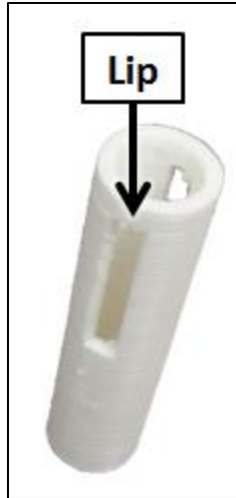
Figure 33: Early prototype of needle cover. Lip indicates where the ridge intended to lock in place broke off.
