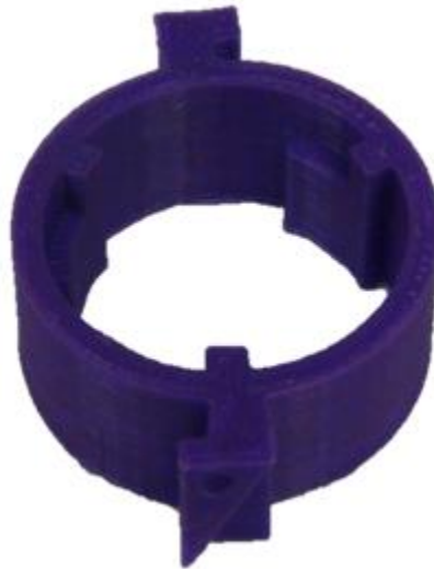
Figure 29: Cylinder Prototype. Cylinder has remained primarily unchanged since the initial design. The dot is used for manufacturing ease due to this parts chirality. The dot belongs on the slot opposite the side of the inner casing with groove.
