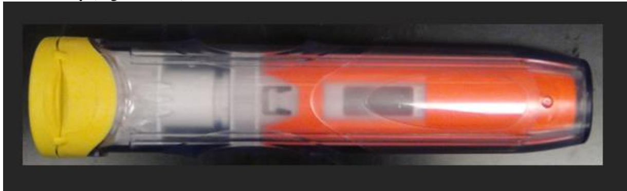
Figure 5: Fully assembled EpiPen® in carrying case , measuring about 6.5” long and 1.5” wide this device is intended to be carried in a backpack or carrying case with a second device close by.
