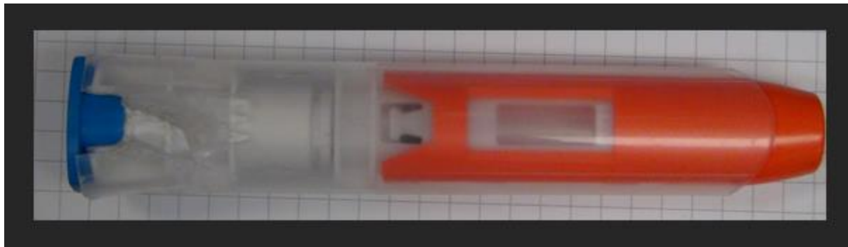
Figure 6: EpiPen® reassembled after being activated , taken apart and reset to appear as it did prior to activation. The distal aspect of the device was torn open on either side to allow the spring holder to be removed from the outer casing. Note how the orange needle protrudes from the proximal end of the device prior to activation.
