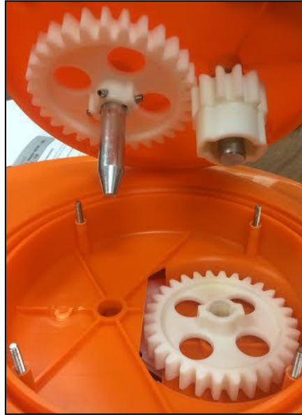
Figure 10 – Salad Spinner with built in gear train.
