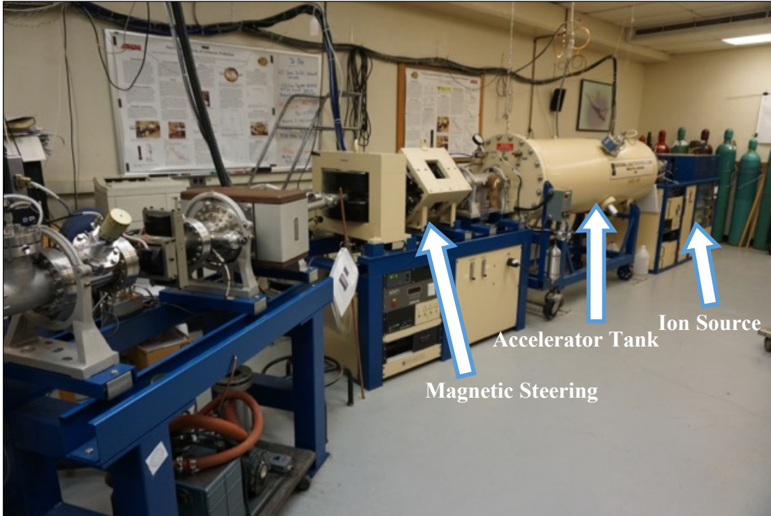
Figure 2: Photograph of the Union College 1.1-MV Pelletron accelerator. Particles originate in the ion source, are accelerated in tandem in the tank, and then are magnetically steered before heading to the scattering chamber shown in Figure 3.
