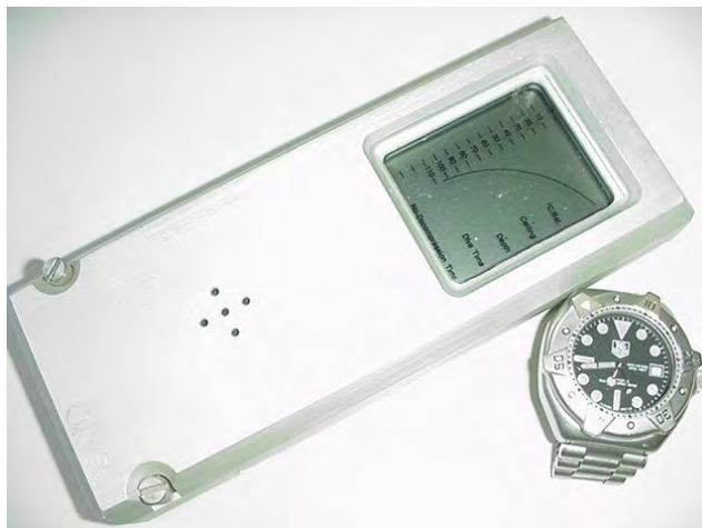
Figure 2: The First dive computer, The Orca Edge, Next to an Early Dive Watch
