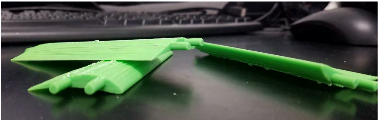
Figure 12: Turbine blades, manufactured through additive manufacturing (3D printing).
