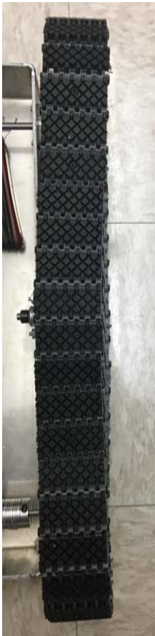
Figure 5.5 – Top and side view of the tread system for the final chassis design
