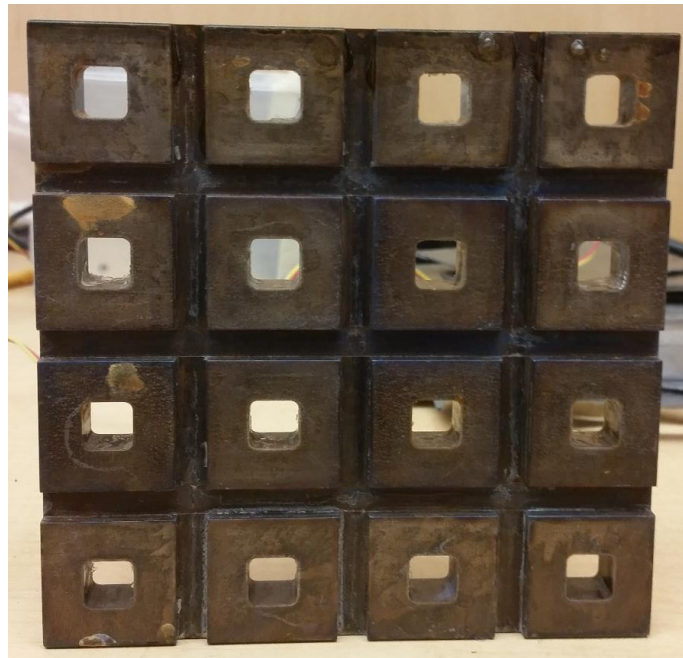
Figure 8: 127 x 127 x 12.7 mm mold, with 16 wells, each 10 x 10 x 12.7 mm.
