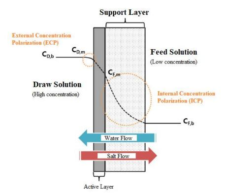
Figure 4. Concentration polarization and reverse salt flux flow in Pressure Retarded Osmosis (PRO).  $C_{D,b}$  and  $C_{F,b}$  draw solution and feed solution concentration respectively.  $C_{D,m}$  shows concentration on active layer and  $C_{F,m}$  shows concentration between active layer and support layer [7].
