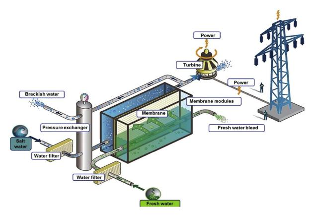
Figure 5. Seawater-river water PRO process for electricity production, adopted by Statkraft [16].
