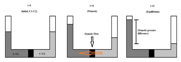
Figure 3. Schematic drawing of pressure retarded osmosis [11].
