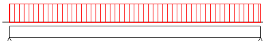
Figure 2b. The set up for the dead load for 1.25 kN
