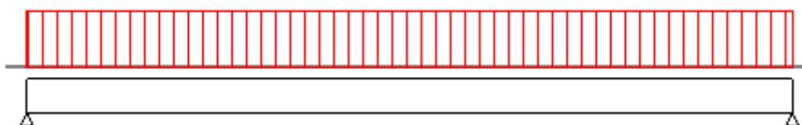
Figure 2a. The initial loading of the system setup for the 1.5 kN
