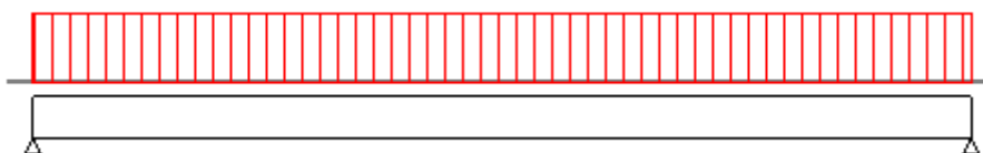
Figure 2c. The set up for the Live load for 1.0 kN
