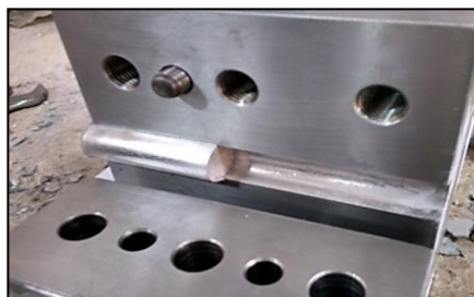
Figure 1. Split die for powder compaction.
