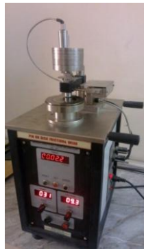
Figure 2. Wear and friction monitor ED-201 with a pin on the disc.
