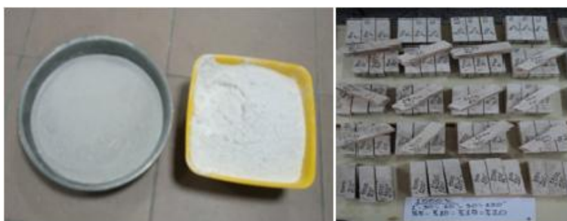
Figure 1. Thermal processed samples with raw perlit-based gypsum binder
