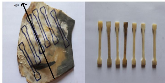
Figure 4: Cutting specimens diagonal to the fibers [4]
