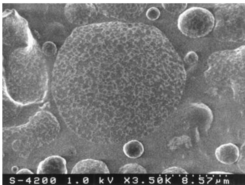
Fig.9 Cryo-SEM for O/W/O emulsion with organoclay
