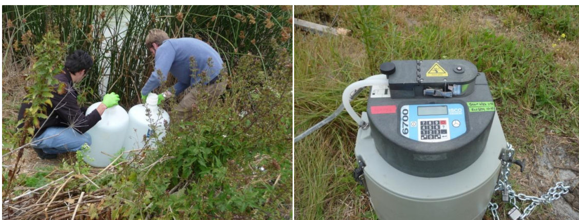
Figure C1. Bromide tracer solution was added over a 20 minute interval at the wetland inlet (left photo). Automated sampling at the outlet using an ISCO 6700 occurred hourly for 7 days (right photo).
