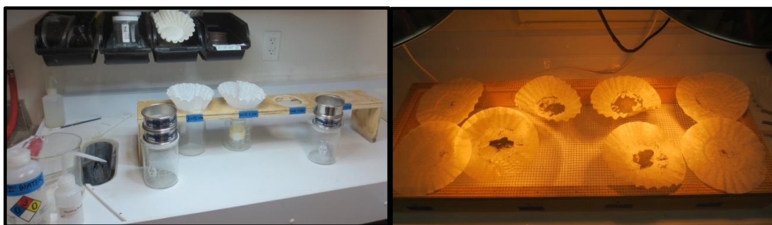
Figure 11. Set up procedure for sieving: stacks, drip bar, and drying screen
