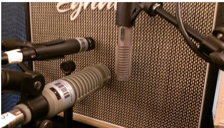
Figure 10: Tracking with an eight-string guitar with a SM57, RE20, R-122, and a E22S
