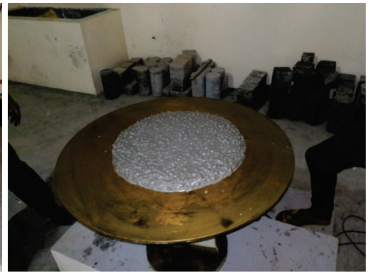
Figure 3 – Experimental Setup of Flow Test
