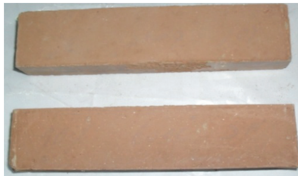
Fig10-Prismatic molds cooked at 850 °C
