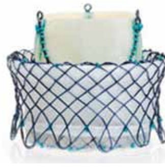
FIGURE 12. The HLT™ valve (Heart Leaflet Technologies Inc., Maple Grove, MN, USA) has porcine leaflets mounted on a self-expandable nickel-titanium alloy wire stent. Additionally, the leaflets are sewn to flexible post to reduce valve and tissue stress.
