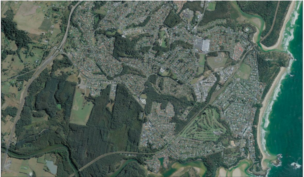
Fig. 26. Geo-referenced 2009 aerial photograph of a portion of the south-eastern sector of the Coffs Harbour LGA. The outline of this aerial photograph exactly corresponds to those of Figs 24 and 25 (1964, 1984) to enable direct comparison. This high-resolution ADS40 photograph is much sharper than the previous monochrome aerial photographs, necessitating an element of careful interpretation to the earlier photographs of the same site. However, what is striking is the change over 45 years from an essentially rural and forested landscape to one of high-density housing with isolated patches of forest dissected by roads. Nevertheless, some Koala habitat is still visible, as are connecting links in the landscape, such as the vegetation bordering Bonville Creek, on the southern boundary of the photograph. This explains why some Koalas would occasionally be seen in urban areas.
