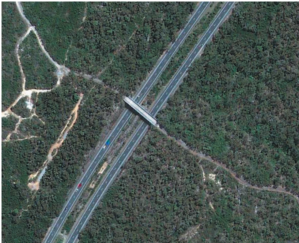
Figure 2. Royal National Park is divided from Heathcote National Park for much of its western boundary by the Southern Freeway. The bridge over the freeway for Cawley Creek Rd (a management road) could be partially converted to a wildlife land-bridge.
