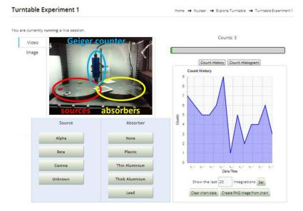
Figure 1: Screenshot (annotated) of the FARLabs 'Turntable' experiment. A live video feed displays the sources, absorbers and the Geiger counter (top left). When the student selects a new source and absorber, the turntables rotate to position them below the counter. The live data feed displays count rate versus time and is updated on a second by second basis.
