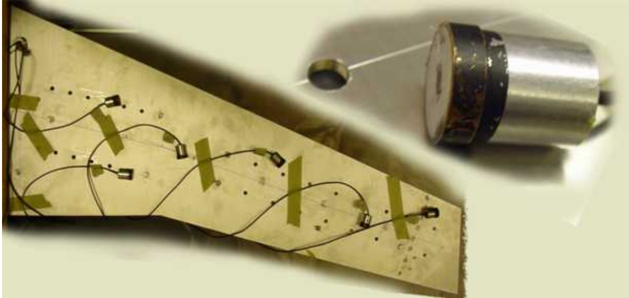
Figure 1. A close up of a swept-back wing where accelerometers are fastened. In the right corner an accelerometer is shown.
