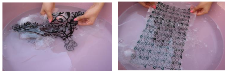
Fig 4 PVA fabric dissolving in water
