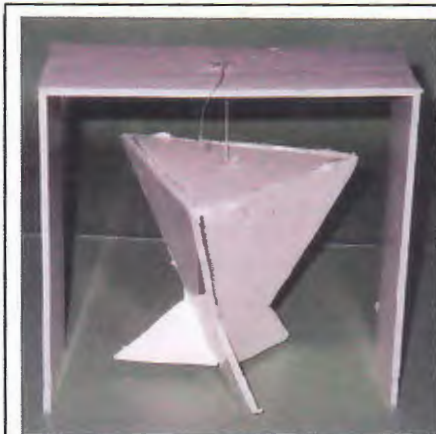
Figure 23. K. N.'s miniature golf obstacle. The symmetric pendulum is hung from the centroid of the triangle. As a result, the obstacle hangs almost perfectly horizontally.
